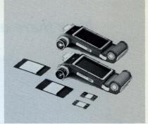
120 ROLLFILM HOLDERS Model A (6 x 9 cm) Cat. No. 60605 Takes (8) 2½ x 3½ exposures. Model B (6x7 cm) Cat. No. 60606 Takes (10) 2½ x 2¾ exposures. Each also takes (12) 2½ x 2½ and (16) 1½ x 2½ shots, and is supplied with viewfinder masks for these sizes. Each attaches directly to camera equipped with Mamiya back, in place of groundglass panel housing.
