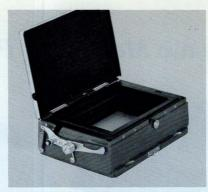
GROUNDGLASS PANEL Cat. No. 00000 Attaches to camera equipped with Mamiya back. Used for viewing and focusing through the lens. Necessary when camera is to be used with sheet film/plate holders or film pack adapter. Groundglass screen is recessed and shielded from overhead light by flip-open cover Quickly detachable when rollfilm holder is to be used. Supplied as standard equipment with Mamiya 23 Deluxe (Cat. No. 60051) available as accessory for Mamiya 23 Standard (Cat. Nos. 60055 and 60056)
